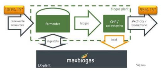
The easiest application is the pre-treatment of biogas digestate. The solid parts of the digestate are mainly composed of cellulose und hemicelluloses which were not available for biogas production. The maxbiogas LX-plant pre-treats the digestate in such a way that it is transformed almost completely into biogas in the biogas plant fermenter. The energy used by the maxbiogas process is supplied by the power generation or by the gas purification of the biogas plant.
